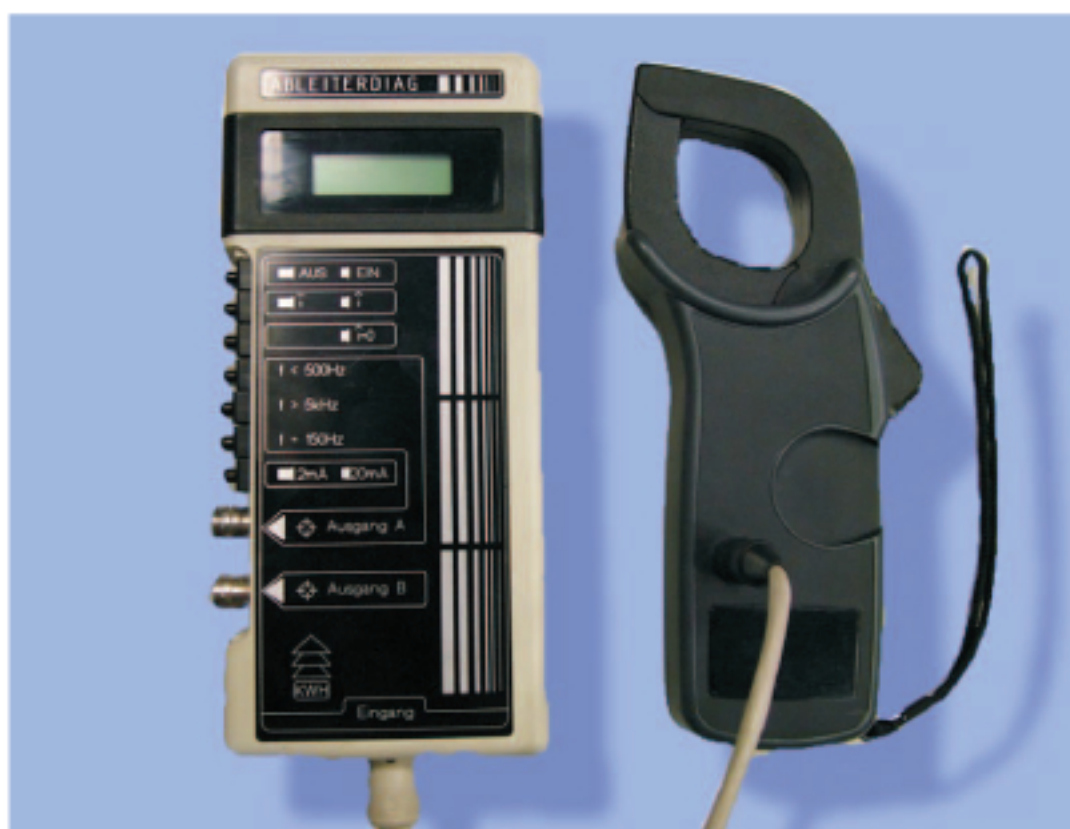
Diagnostic Appliance for Current Analysis of Metal-Oxide-Arrester
